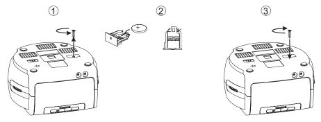
If the power is interrupted the clock display will go off but the battery will maintain the Time, Alarm time and Radio preset stations settings. When power is restored the time display will be correct and the alarm time and preset radio stations will also be maintained.
